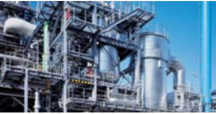
▲ Diphyl® flash system with a total output of 20 MW at 360^{\circ}\text{C} supplying process heat to a DMT plant in Germany.
